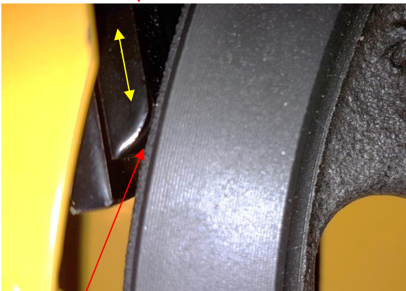
Free position. Position of the belt brake. The coupling plate contacts the large pulley. NB! clutch movements as big as possible.
