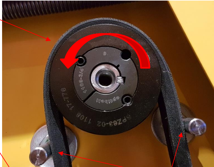
Free position. The belt should be free from the pulley. Contact pins/belts in free position.
