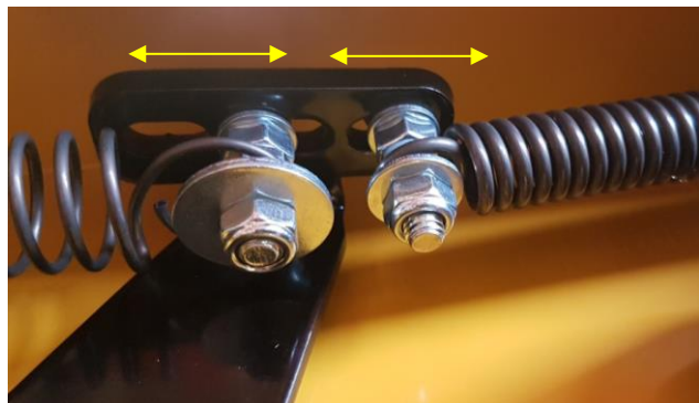
Adjusting the springs can tighten the belt.
